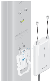
Mounting on a Sector Antenna
